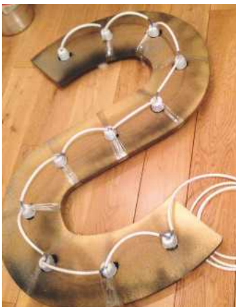
▲ Pic.12 Once all the holders were safely wired, it was time to fit them. This was done using some Sugru and some Sellotape to hold them in place while the Sugru cured
